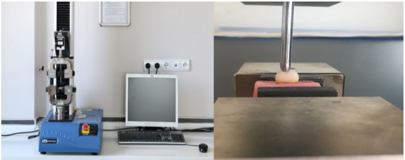
Fig. 2. Fracture strength set-up
