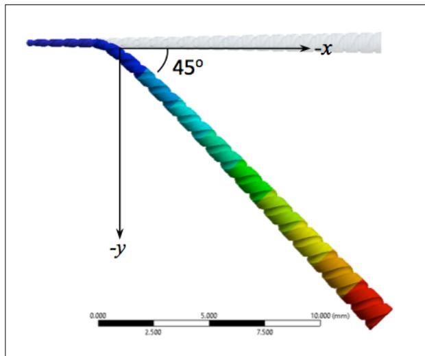
Fig. 3. 45° displacement in -y axis to the endodontic file model.
